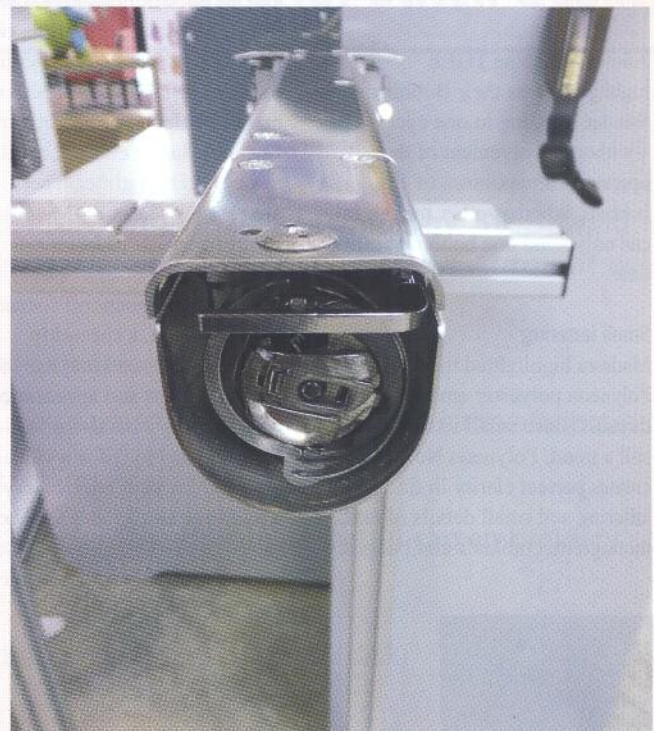
● The tubular arm of the Sprint 6 works without a picker at the front.
